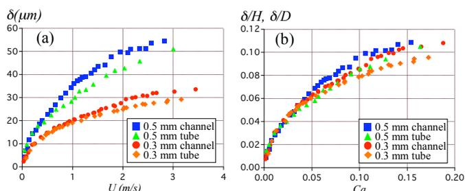
Fig. 6 (a) Thickness of liquid film against velocity (b) Dimensionless thickness against Capillary number
