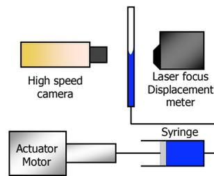
Fig. 1 Schematic diagram of experimental setup
