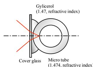
Fig. 3 Schematic diagram of micro tube
