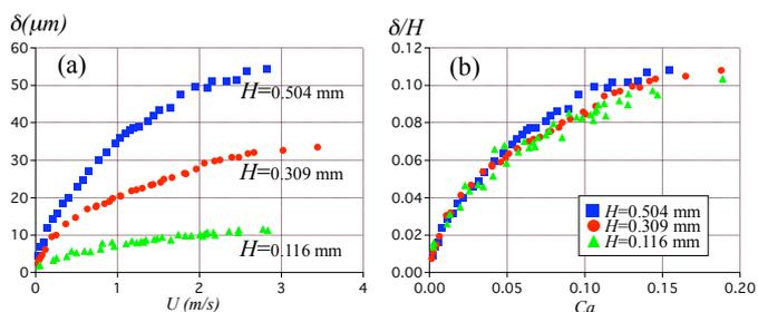
Fig. 5 (a) Thickness of liquid film in micro channel against velocity (b) Dimensionless thickness against Capillary number
