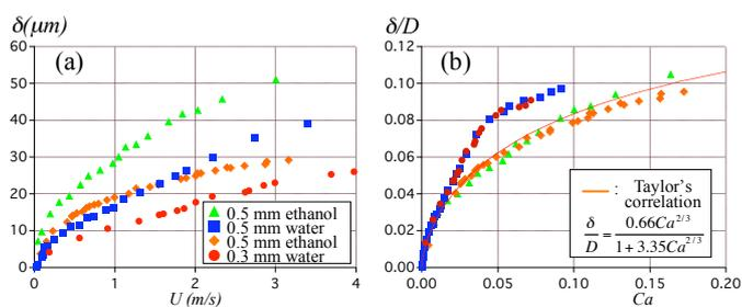
Fig. 7 (a) Thickness of liquid film against velocity (b) Dimensionless thickness against Capillary number
