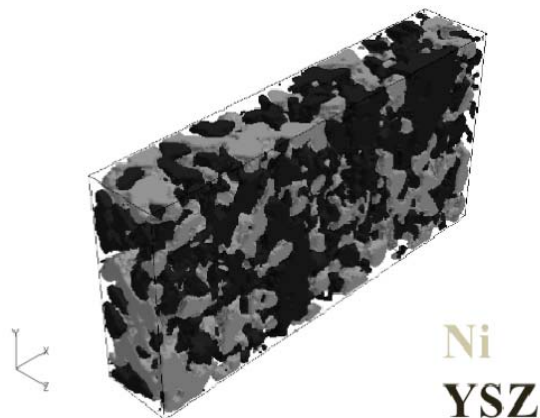
Fig. 3 Three-dimensional re-constructed anode of an SOFC
