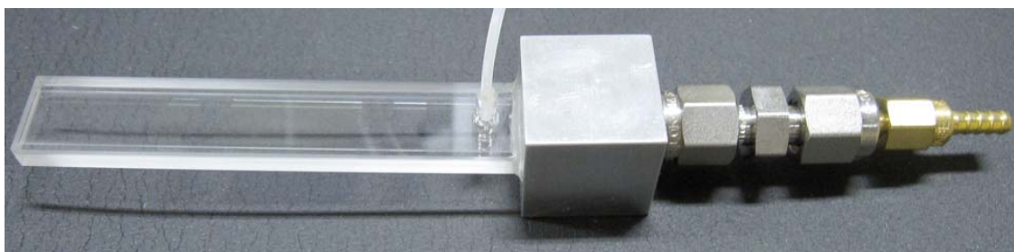
Fig. 2 Aluminum block connected to the high aspect ratio rectangular channel.
